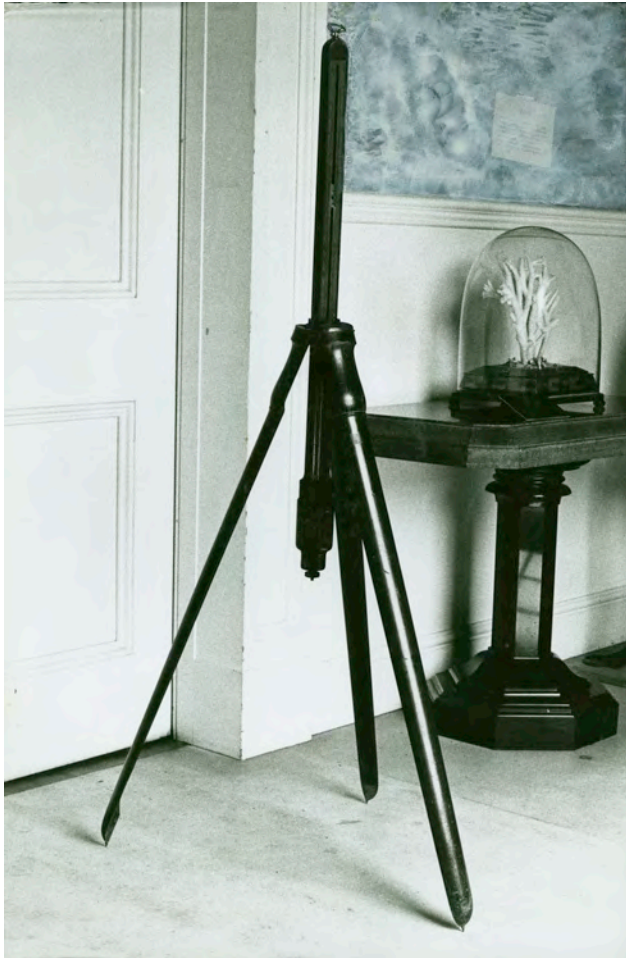
Figure 16.2: Portable Barometer. Photograph by the authors at Chatsworth. This is probably the barometer that Cavendish carried to the top of Garth Mountain to measure its height. When folded into its mahogany case, the barometer measures 43\frac{1}{2} inches. The instrument is suspended in gimbals. At the bottom, near the wooden cistern, there is a thermometer with a corrections scale. William Roy, with whom Cavendish collaborated on experiments with barometers, used a portable barometer almost identical to this one for taking heights of mountains. Although the Chatsworth barometer is unsigned, we know from Roy that this kind of barometer was made by Jesse Ramsden. Roy (1777, facing p. 658). The photograph is reproduced by permission of the Chatsworth Settlement Trustees.
