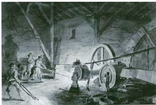
Figure 16.3: Working Iron at Merthyr Tydfil. Watercolor by J.C. Ibbetson in 1792. A mass of hot iron is being struck by a trip hammer to remove slag. Courtesy of Cyfarthfa Castle Museum.
